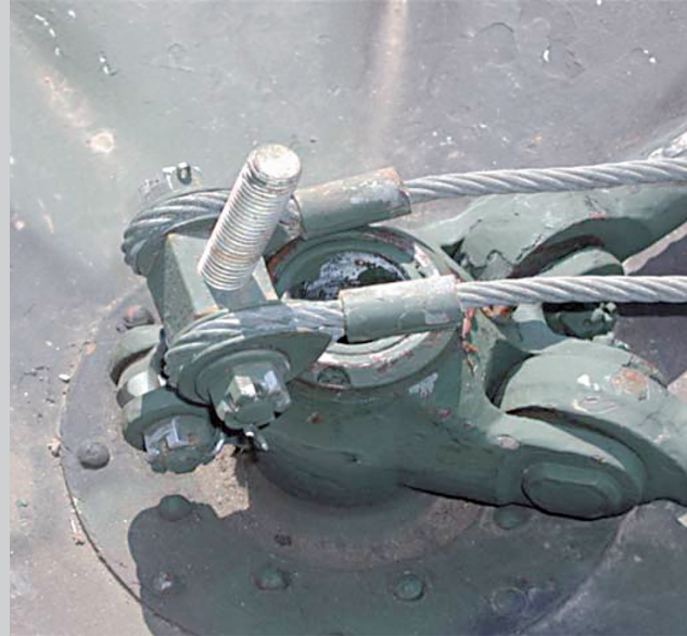
Fig. 4 — AlumiPlate™ after 22 months of sea exposure.
