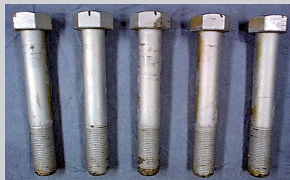
Fig. 2 — AlumiPlate™ after a 2500 hour salt spray test in accordance with ASTM B117 .
