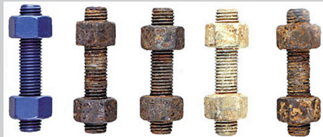
Fig. 1 — Comparative results of a 1000-hour salt spray test performed in accordance with ASTM B117 .
